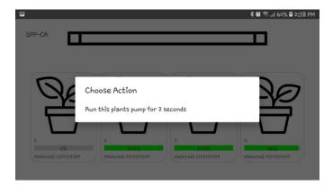
When you click the "Run this plants pump for 2 seconds" text, the pump will run for that plant. This allows you to ensure you have the correct pump on the correct moisture sensor. It also allows you to run the pump while you position the water hose outlet to where you want the water to be applied.
