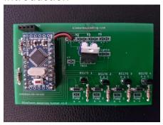
PlantMate is an Arduino based automatic plant watering system that can maintain up to 4 plants. This system includes the PlantMate circuit board with a 6V power adapter, 4 water pumps (hoses not included) and 4 moisture sensors.
